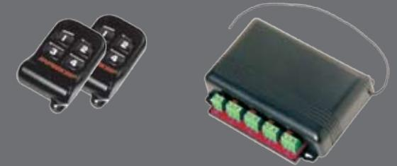
The "Enforcer" add-on module can be connected to the GUARD8 switch lock to arm and disarm the system remotely and can also be used to activate the audible panic function.
