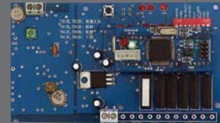
The Four-Zone Wireless Receiver can be fully integrated with the GUARD8 Security System to allow for the use of wireless PIR sensors and magnetic door contacts, but is so versatile that it can be incorporated in most existing alarm installations.
