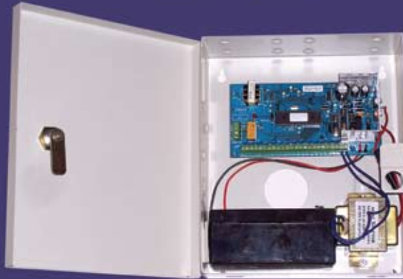
CONTROL PANEL & BACKUP BATTERY
